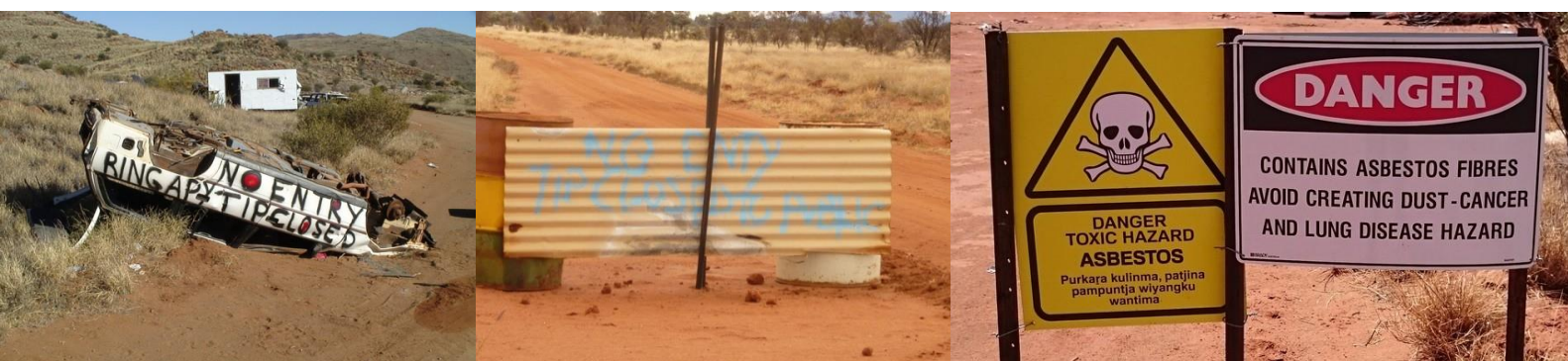
Figure 5.4 – Examples of temporary and permanent hazard signs
