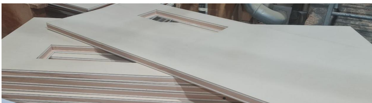
Figure 4: Partially completed fire doors with the FRBs sealed within.
