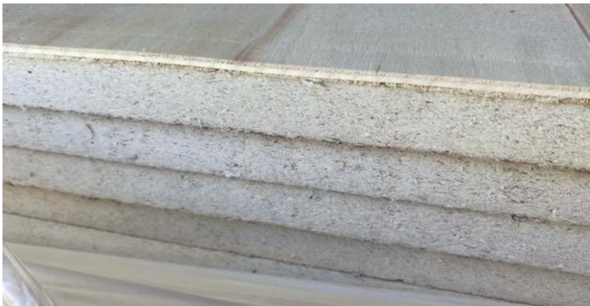
Figure 1: End view of FRBs with composite construction visible. Plyboard used for transport.
