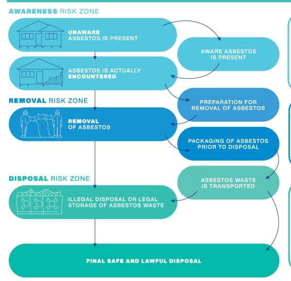
Risk of exposure to asbestos fibres if ACMs are accidentally disturbed. Absence of planning in this zone leads to significant risks in later zones.
