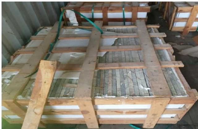
Figure 3: Imported cut stone tiles from India described as Bidasar Green and Bidasar Brown 'marble' found to contain asbestos.
