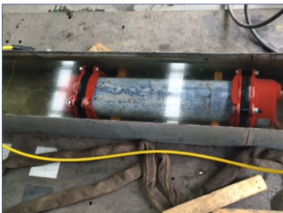
Photo (left): Exhumed cured in place samples that were extracted to be laboratory tested.
