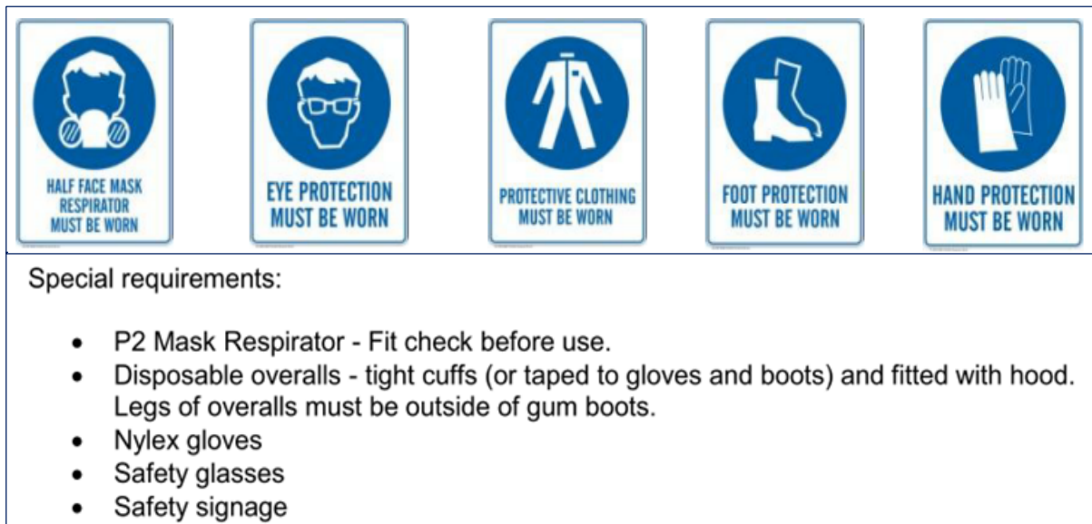
Figure 4.1: PPE that must be worn, and special requirements that must be complied with, when cutting AC pipe or in the vicinity of cutting of AC pipe.
