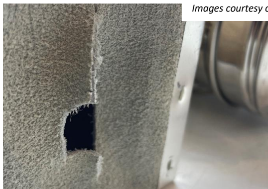
Figure 3: Bellows material cut for analysis
