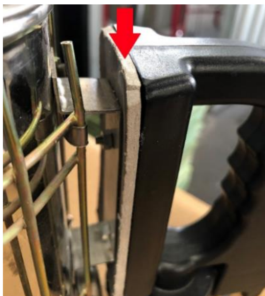
Figure 5: Insulation board indicated
