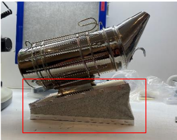
Figure 1: Manual bee smoker – bellows indicated
