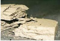
**FRIABLE:** flaky, powdery, can be broken up easily with your fingers; or due to a work process, the asbestos material becomes such that it may be crumbled or reduced to powder by hand pressure. Can be found in loose-fill insulation and pipe lagging. It is extremely hazardous because the fine asbestos fibres can be easily released into the air and inhaled.
