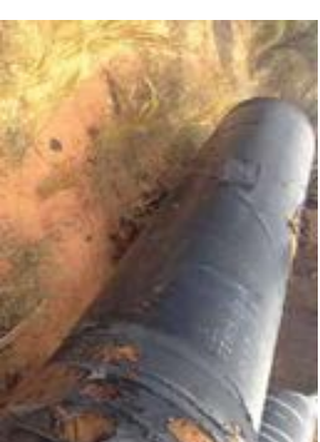
Figure 24 and 25: The redundant pipes were in varying states of degradation
