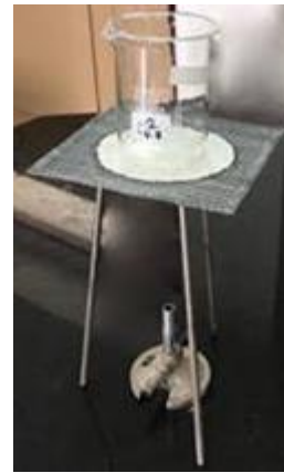
Figure 2: Gauze mat sitting on tripod over Bunsen burner. (Ref: Health and Safety Executive, United Kingdom)
