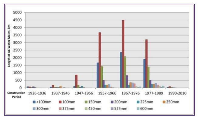
Figure 1 AC water mains by diameter and construction period (from WSAA 2013)
