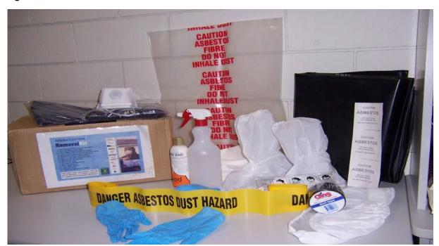
Figure 8.3 – Latrobe asbestos in the home removal kit
