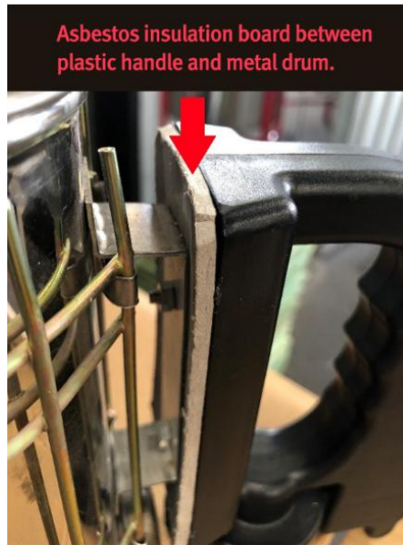
Figure 2: Close-up of asbestos containing insulation board. (ref: Workplace Health and Safety Queensland)
