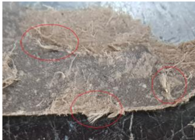
Figure 5: Deconstructed RC engine gasket material showing asbestos bundles present - Image source: Lifetree Environmental Pty Ltd
