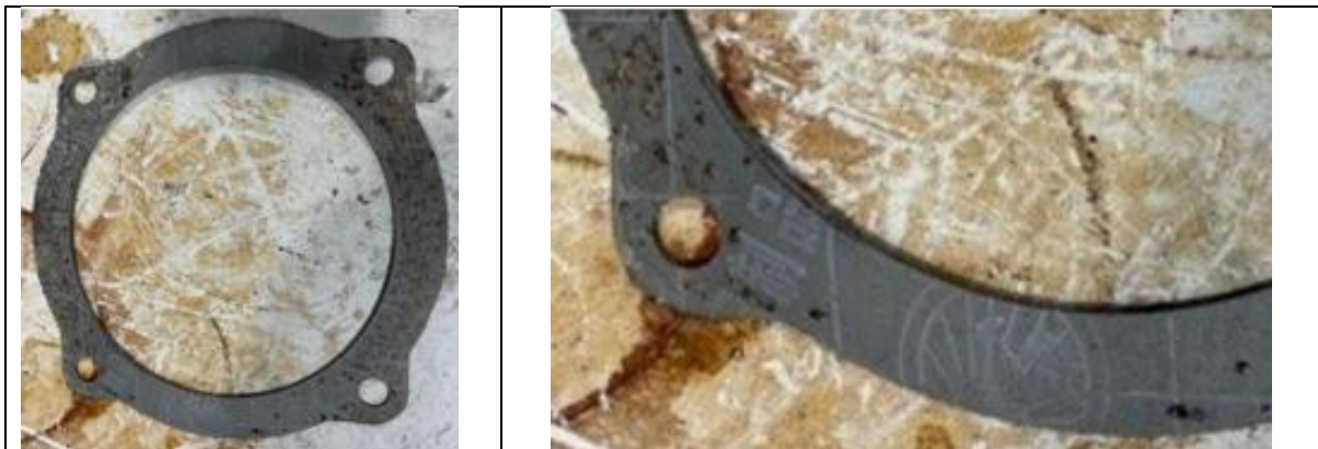
Figures 4 and 5: Chinese origin gasket with asbestos showing manufacturer markings.
