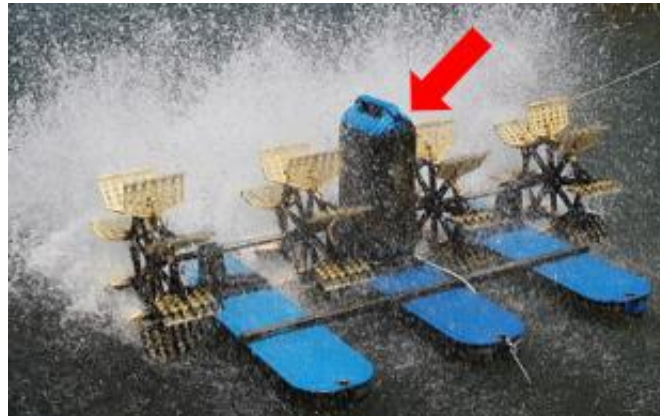
Figure 1: A paddlewheel aerator in use. Arrow indicates motor and gear reducer, under housing.
