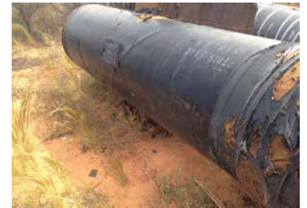
Figure 24 and 25: The redundant pipes were in varying states of degradation
