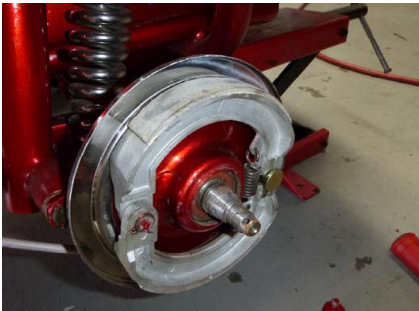
Photo 1: Sidecar brake pads (containing asbestos) removed from imported Vespa scooter.
