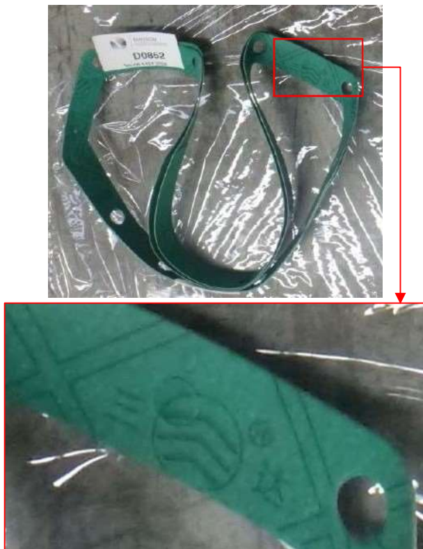
Figure 2: After-market gasket 144-33-21340 with markings.
