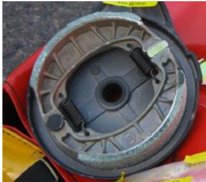
Photo 1: Brake Pads (containing asbestos) and drum assembly removed from imported electrical scooter.
