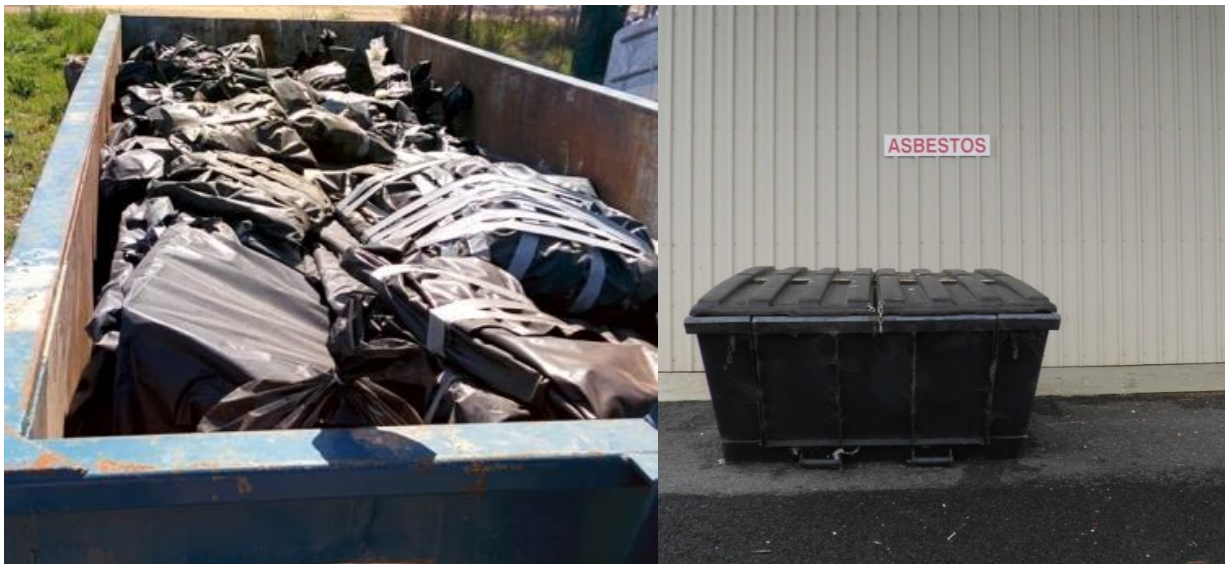
Figure 12: Asbestos disposal facilities at transfer stations in Victoria (left) and Tasmania (right)
